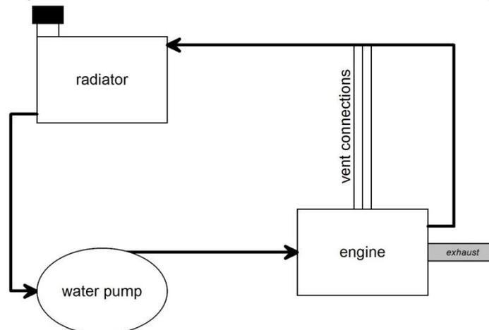
4. Note the positions of the in- and outlets, route and attach the hoses properly and ensure that there are no kinks or sharp bends in the hoses.
