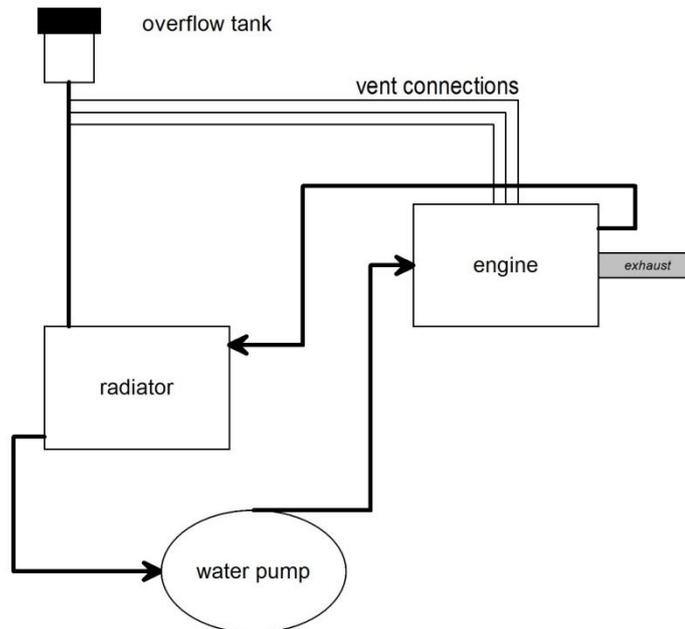
4. Note the positions of the in- and outlets, route and attach the hoses properly and ensure that there are no kinks or sharp bends in the hoses.
