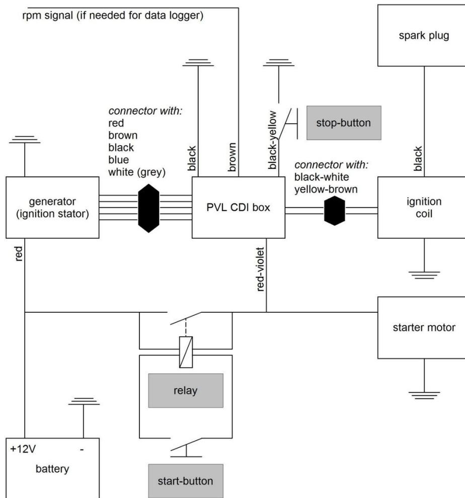
↪ Use sufficiently big cables for the conductive circuit between battery, relay and starter motor ( $10\text{mm}^2$  / AWG8).  $1.5\text{mm}^2$  / AWG16 cables are sufficient for the control circuits.
